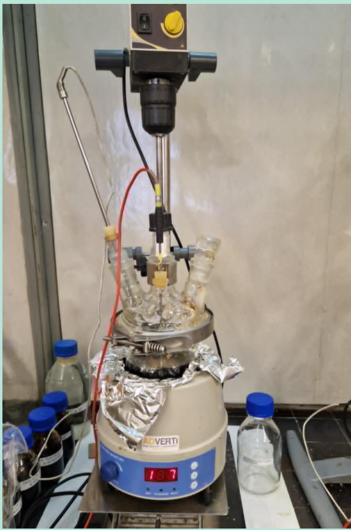
Fig. 1. Apparatus for PUR foam glycolysis reaction.
